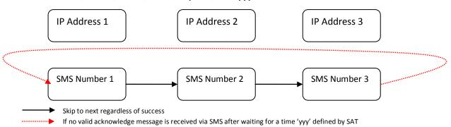
Diagram above illustrates the case when all three slots for SMS numbers are filled although there are no restrictions. If any of the SMS number locations is left empty, flow stops sending reports at that location and starts to wait for acknowledge message for the duration of time defined by SAT.
