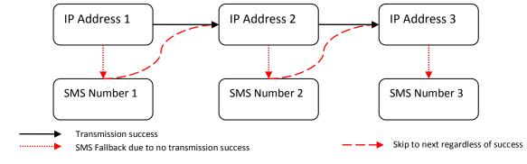
Diagrams above illustrate the case when all three slots both for SMS numbers and IP addresses are filled although there are no restrictions on how many of the available slots are needed to be filled or filled equally with respect to the other row. For the conditions in the first diagram, if any of the IP address is left empty and SMS fallback occurs and at least one SMS number is defined, flow falls back
