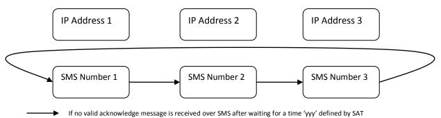
Diagram above illustrates the case when all three slots for SMS numbers are filled although there are no restrictions. If any of SMS number locations is left empty, flow goes back to the beginning as it is the last number in the loop.
