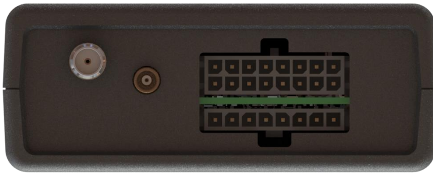
SRT341 side view. From left to right: GSM/LTE antenna, GNSS antenna, Control A (top) and Control B (bottom) interfaces
