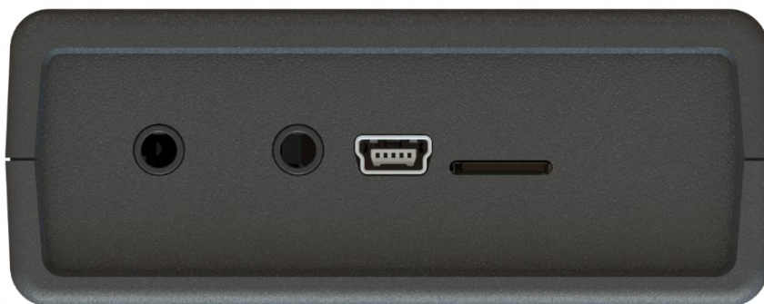
SRT341 side view. From left to right: Mic in, Speaker out, mini USB and SIM card holder
